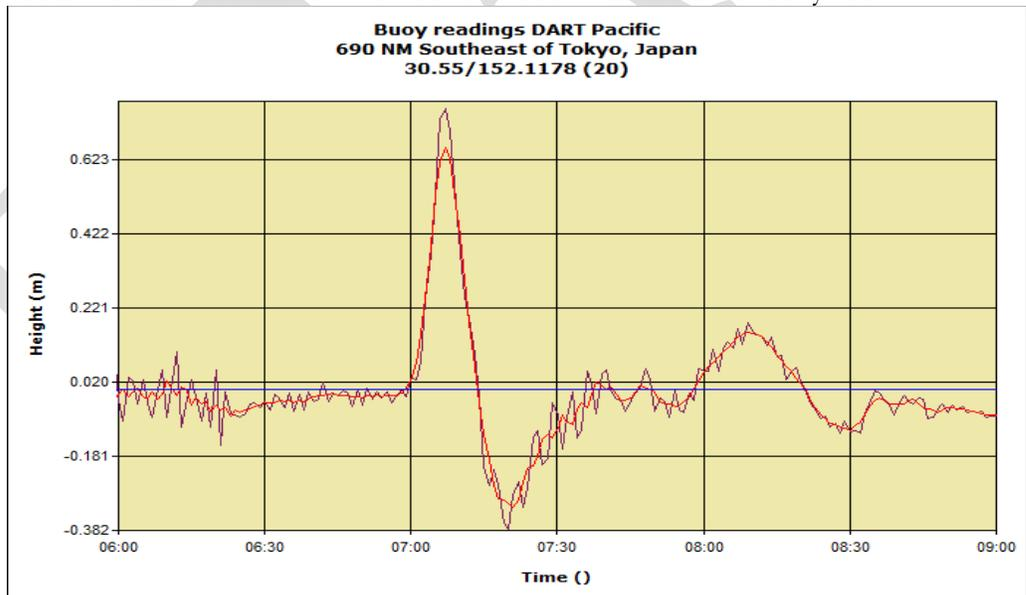
FIGURE 10 – Use of post average averaging procedure (brown curve is with 100 points of Moving average while the in the red curve the residual has been further averaged with 10 points).
