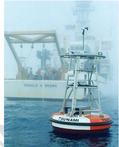
FIGURE 20 – The first operational DART® buoy system design is shown in the photograph on the left (NOAA web site)
