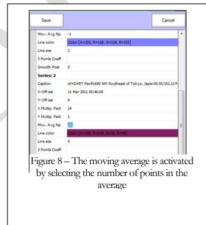
Figure 8 – The moving average is activated by selecting the number of points in the average
