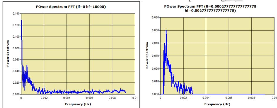
FIGURE 14 – Power spectrof of the curve: left without filtering, right filtering high pass filter at 1h (0.00027 Hz) and 6 min (0.0027 Hz) as low pass filtering
