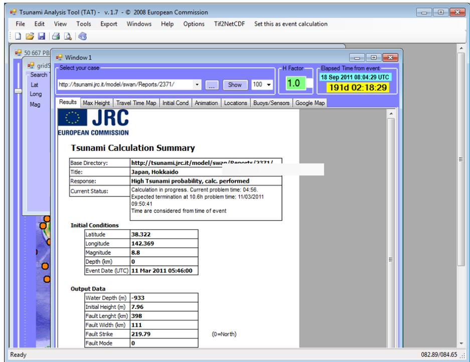
FIGURE 1 – Initial screen showing the characteristics of the calculation
