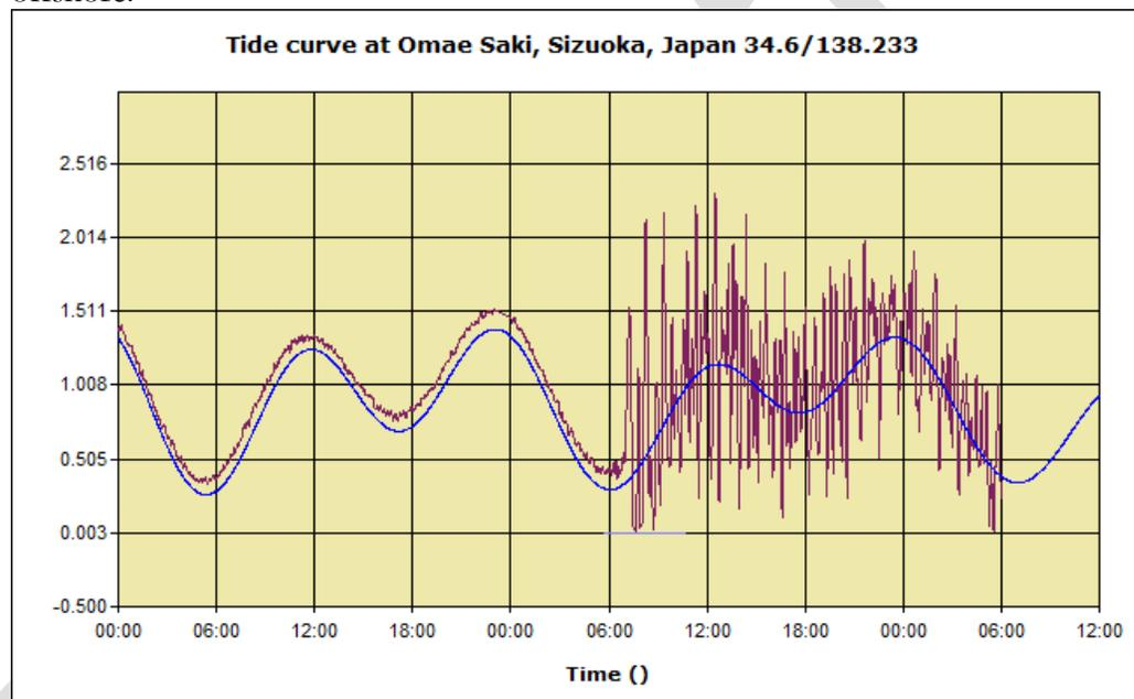
FIGURE 16 – The brown curve is the real signal and the blue curve is the calculated tide
