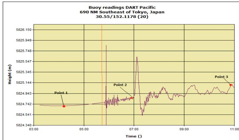
FIGURE 11 – The real curve with the indication of the 3 points that will be selected for the polynomial curve
