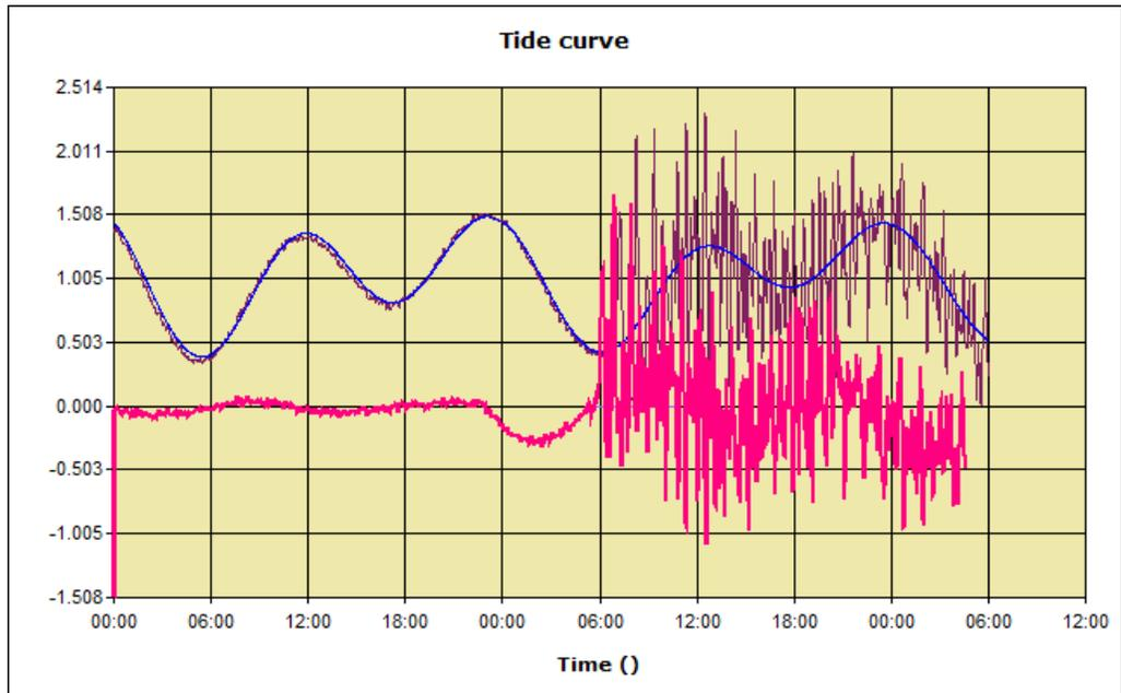
FIGURE 17 – The brown curve is the real signal and the blue curve is the calculated tide corrected with the 2 points procedure while the pink curve is the residual, the difference among the two curves.
